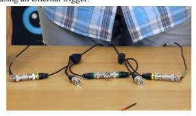
Connect LEMO plugs of LTC-OUT cables and genlock BNC connector to the appropriate sockets of the Ambient Lockit.
