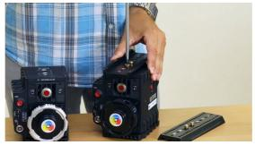
Then to the upper right edge of the camera tighten the motor holders of the follow focus unit.
