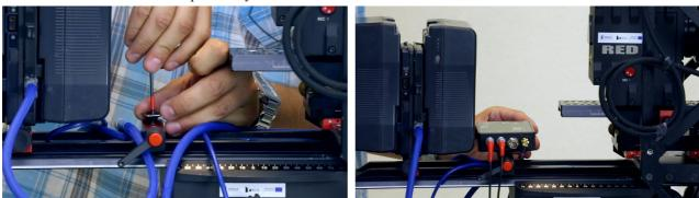
Screw Ambient connector to the previously mounted bracket.
