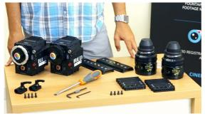
First we have to replace the RED cameras radiatior cover with the Easy Top plates.
