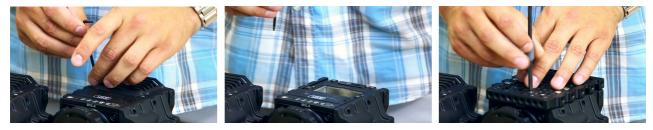
The next stage is to mount CinemaVision camera mounting plates on both cameras.
