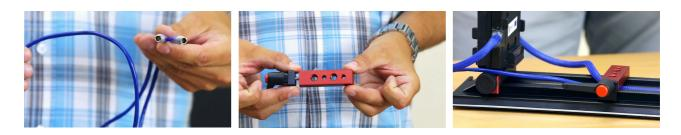
We screw the main mounting plate with the Rig by using three brass screws and a flat-blade screwdriver. The cables can be hooked for a while so as not to interfere.
