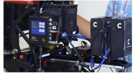
Plug lens motors control cables into the appropriate sockets of the Aladin driver.
