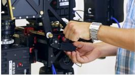
Using the magic arm coupler attach to the Rigs body the Aladin Mark II Follow Focus control device.
