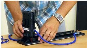
Place camera communication cable GIG-E on the main mounting plate. This cable and the bottom camera power cable should be placed precisely and held with a screw clamp which we will use later to mount Ambient Lockit device.
